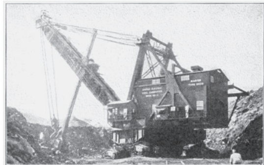
Fig. 103.—Caterpillar-type long-boom power shovel. (Courtesy of the Marion Steam Shovel Company.) The bucket capacity is 23 tons or 20 cubic yards. Vertical sweep of shovel is 82 feet 6 inches. It is estimated that 1,500 men working with picks and shovels would be required to duplicate the work of this one machine. Accident exposure to the operators and ground men who serve this shovel is considerably less than if they and others were obliged to excavate this material by manual labor.
