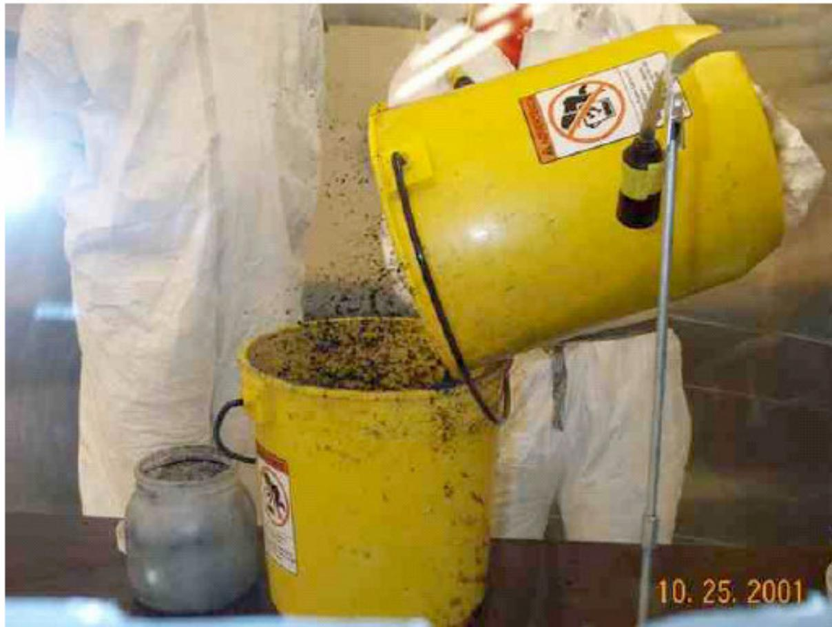
Raw single walled nanotube material
